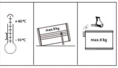
Load capacity depends on weight distribution and handling and decreases with dynamic loading.
