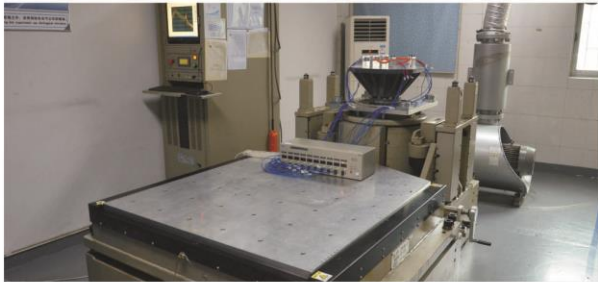
Vibration Test Equipment
